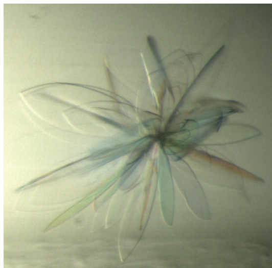
Figure 1 Native crystals of FH-678 402H . Average crystal dimensions were approximately 200 × 50 × 5 µm.
